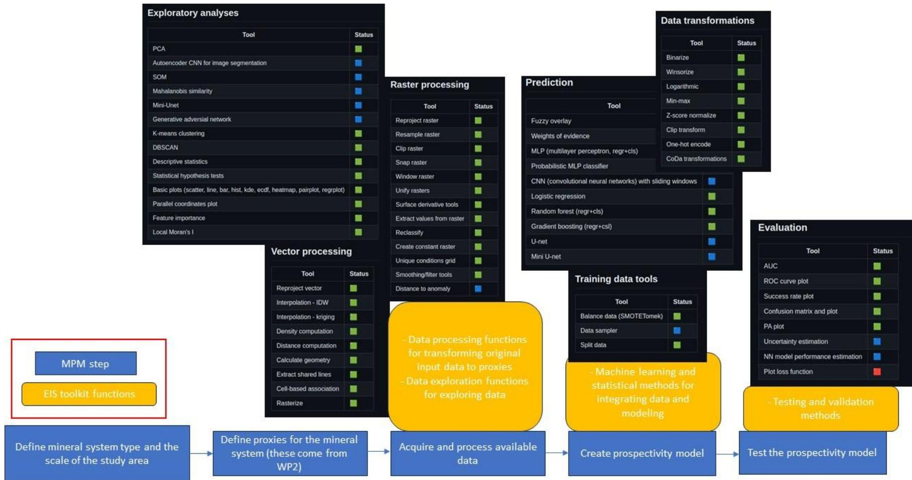
Figure 1. The mineral prospectivity modelling (MPM) workflow (blue boxes) and EIS toolkit functions related to each phase of the workflow (black boxes). Yellow boxes provide a general description of tools needed in each phase of MPM.
