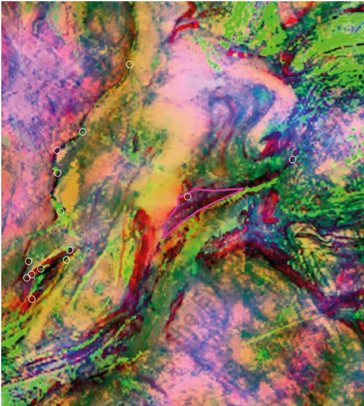
Figure 4: An example subregion (pink) that is similar colour to the known ore deposits (white rings) has been digitized, and its values from bands 1 and 2 have been plotted on figure 5 along with the values of all the data. The data is PCA from multiple geophysical data sources, where principal component (PC) 1 is assigned to red, PC 2 to green and PC 3 to blue.
